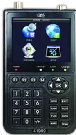
The DTT channel signal power and signal quality may be displayed on the LCD screen after you have configured your local DVB-T parameter. It can also display five channel signals is the same menu, which is very helpful when adjusting the aerial for different multiplexes. It can also supply power to a masthead amplifier, thereby avoiding the necessity to have the download connected while setting the aerial.
